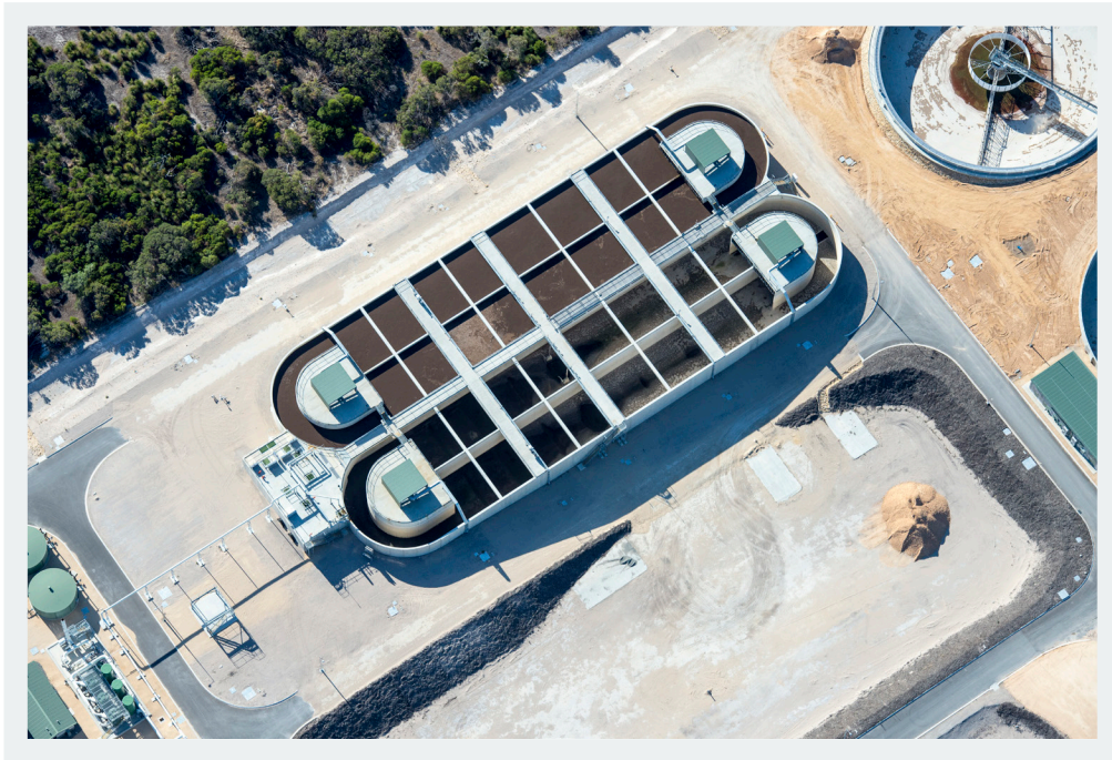
DBS Racetrack OXIDATION DITCH
