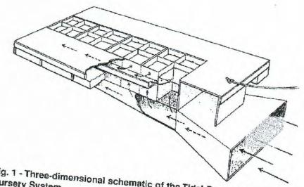
Fig. 1 - Three-dimensional schematic of the Tidal-Powered Upwelling
